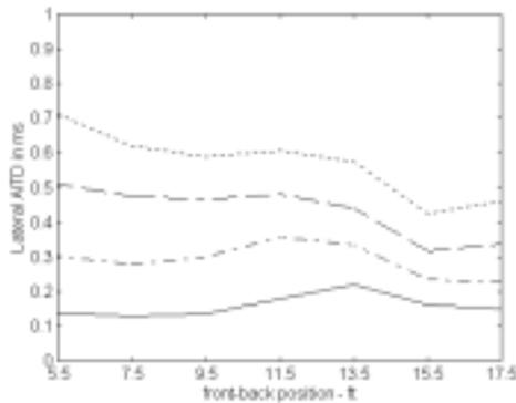
Figure 34: AITD in the range of 30-90Hz along the center line of a 17'x23'x9' room with four drivers, the right side of the room lagging the left side by a variable phase shift.
