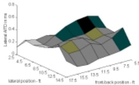
Figure 6: Lateral AITD in the 63Hz octave band for a 17'x23'x9' room, surface reflectivity 0.8. Note the value is lower than in the free field.
