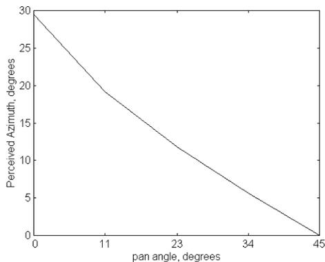
Figure 20: Perceived angle, as calculated from the ITD, for a listener at the ideal listening position, with loudspeakers  $\pm 30$  degrees, as a
