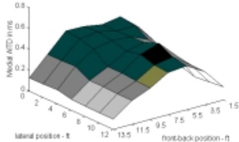
Figure 14: Medial AITD for the 12'x15'x9' room over the 20Hz to 90Hz range. Single driver is in the upper left corner. This picture represents the lateral AITD if the room is set up with the primary listening axis parallel to the short walls, rather than parallel to the long walls. Notice that in this room setting the axis parallel to the short walls gives a much larger lateral AITD than setting it parallel to the long walls. The difference is highly audible.
