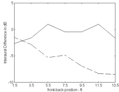
Figure 2: DFT along the center line for the two configurations in figure 1. \_\_\_ = two drivers at the sides of the listener \_\_\_\_\_ = two drivers at the front. Note the approximately 5dB difference in envelopment in the listening area.
