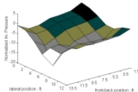
Figure 11: The Normalized Average Pressure in a 12'x15'x9' room in the 63Hz octave band from a single driver in the top left corner.
