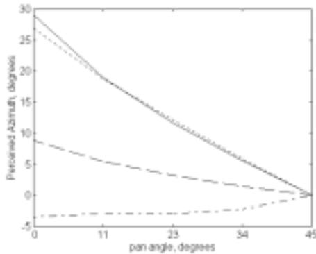
Figure 22: Pan law for four different room reflectivities. \_\_\_ = anechoic, - - - = 0.5, \_\_\_ \_\_\_ = 0.65, - . - . = 0.8. Note the ability to localize horizontally goes down rapidly as the reflectivity goes up. Same room and positions as figure 21.
