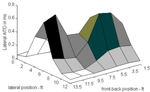
Figure 12: Lateral AITD in a 12'x15'x9' room, surface reflectivity 0.8, single driver in the top left corner, 63Hz octave band. This band has the largest AITD for this speaker position in this room. The next figure is more typical.
