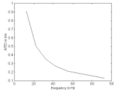
Figure 24: The dependence of the AITD in the center of figure 22 with frequency. Note the typical values of 0.2ms or so above 60Hz. Adding surface reflections can increase this value.
