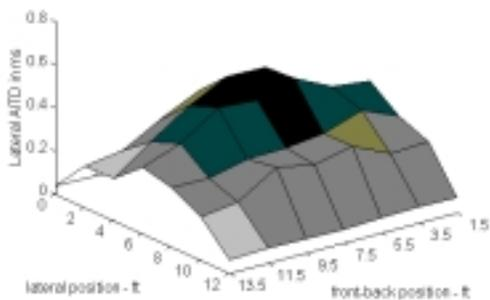
Figure 16: The Lateral AITD over a range of 20Hz to 180Hz in a 12'x15'x9' room with the driver at the side. Note the significantly higher values than for figure 13.
