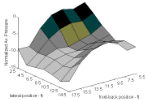
Figure 10: Normalized Average Pressure in the 63Hz octave band from a single driver of unit strength in the upper left corner of a 17'x23'x9' room. The wall reflectivity is 0.8. Note the pressure in the listening area is low. Equalization can raise the pressure, but it cannot change the AITD.
