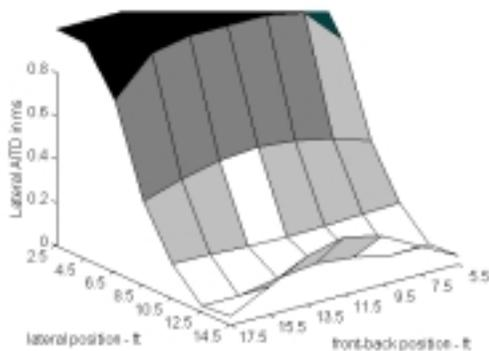
Figure 23: Lateral AITD in an anechoic space, two drivers on opposite sides of the listener, separated by  $\pm 11'$ . Left driver leads the right driver in phase by 90 degrees. 22.5Hz. Note the peak in AITD at  $-4'$  from the center, and the minimum at  $+4'$ . These values correspond to the minimum and maximum in the pressure response. The value of AITD along the center axis ( $8.5'$ ) depends on the spacing of the minimum and maximum.
