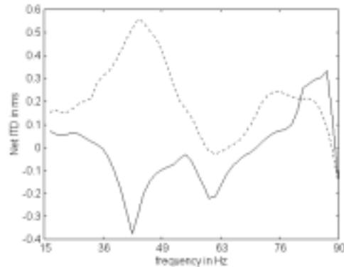
Figure 21: The frequency dependence of the ITD as a function of frequency for a single driver at  $x=-.5'$ ,  $y=.1'$ ,  $z=1.5'$  for a listener at  $x=6'$ ,  $y=9.5'$ ,  $z=4'$  in a  $12' \times 15' \times 9'$  room with reflectivity 0.8. — = lateral ITD. - - - = medial ITD. Note that for frequencies below 70 Hz the lateral ITD is negative, and the speaker appears to be in the opposite corner.
