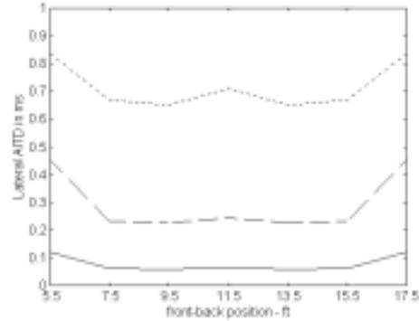
Figure 30: The Lateral AITD in the 63Hz octave band for the same configuration as figure 28. The AITD for the 90 degree shift is again moderate, the 30 degree case is much too low, and the 150 degree case is too high. Note that for this frequency band the AITD for 90 degree phase is approaching the anechoic value. The value below 50Hz and above 70Hz is ~0.4ms.
