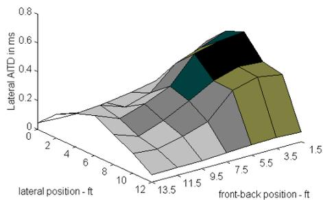
Figure 13: The Lateral AITD over a range of 20Hz to 90Hz in a 12'x15'x9' room from a single driver in the front left corner. Surface reflectivity is 0.8.
