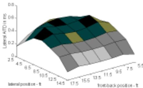
Figure 18: The Lateral AITD over a range of 20Hz to 90Hz in a 17'x23'x9' room with the driver at the side of the room in position  $x=0.1'$ ,  $y=11.5'$ ,  $z=1.5'$ . Note the substantially higher values than for figure 17.
