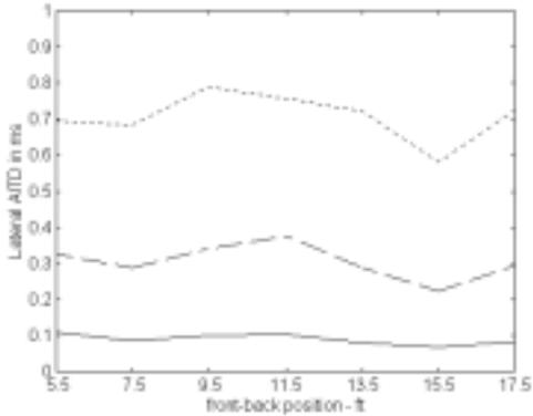
Figure 28: The lateral AITD in the 63Hz octave band along the center axis of the same room. \_\_\_\_\_ = 30 degrees, \_\_\_\_\_ = 90 degrees, - - - = 150 degrees. Note the very low AITD for the 30 degree case, and the moderate AITD for the 90 degree case. The 150 degree case is unnaturally large and phasy.
