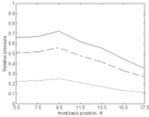
Figure 27: The Normalized Average Pressure along the center axis of the room from figure 25. \_\_\_\_\_ = 30 degree shift, \_\_\_\_\_ = 90 degree shift, - - - = 150 degree shift. Note the ~3dB reduction in pressure in the 90 degree curve.
