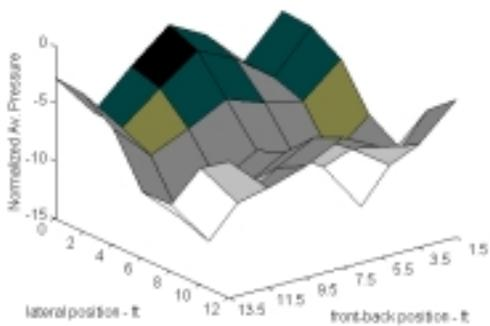
Figure 15: Normalized Average pressure in the same room, but the driver is now at the side of the room, at  $y=7.5'$ ,  $x=0.1'$ ,  $z=1/5'$ . Although the driver is not in the corner of the room, the pressure in the listening area is not significantly reduced. See figure 11.
