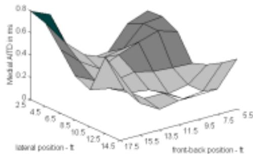
Figure 7: Medial AITD for the same room. Note the value is larger than figure 5, but still
