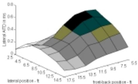
Figure 17: The Lateral AITD over a range of 20Hz to 90Hz in a 17'x23'x9' room with the driver in the upper left corner. See the pressure response in figure 10.
