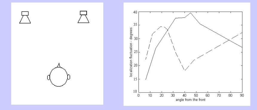
Hearing envelopment depends on <u>differences</u> in the signals between the ears. The difference depends on frequency. At about 1500Hz the front speakers will sound as if they are at the sides if the signals are decorrelated. Thus standard stereo can be enveloping even without the room - but only above 1000Hz!
