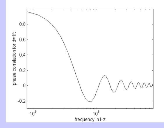
Correlation between two omnidirectional microphones separated by 25cm in a reverberant field. Note the high correlation at 200-300Hz, and a negative correlation at 800Hz. Small distances are not sufficient for decorrelation!
