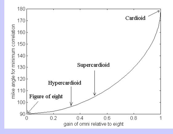
Reverberation is decorrelated in a microphone pair if the mike angle is correctly chosen. These angles are generally also optimum for the front image.
