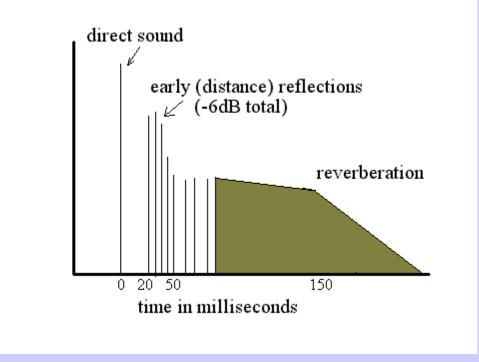
A strong early lateral field gives the sound distance and an acoustic integration. Reflections in the range of 50 to 150ms are minimized, while keeping reflections after 150ms strong.
