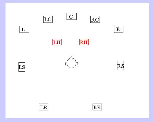
Ideally  $\sim 11$  loudspeakers could be used - 5/4 with two overhead speakers
