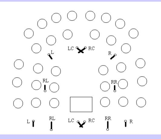
Two supercardioid pairs are used for the center of the ensemble. They are mixed left-to-center and right-to-center. Four cardioid microphones point rearward, in front and behind the conductor. These create the rear channels.
