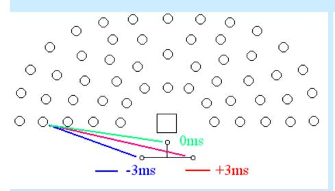
Record the orchestra with a "Decca Tree" - three omni microphones separated by one meter. A source on the left will give three outputs identical in level and differing by time delay.
