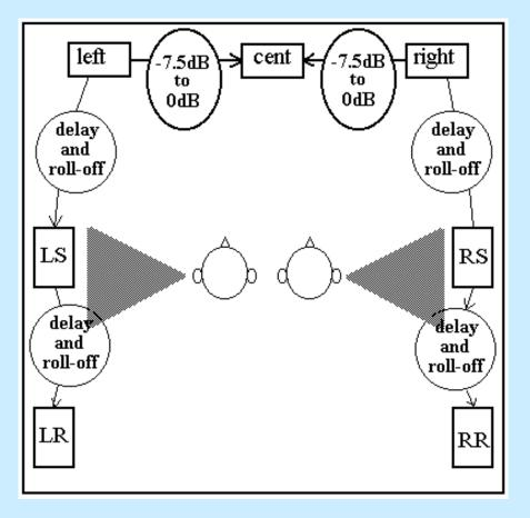
Diagram shows matrix decoding with NO directional steering.
