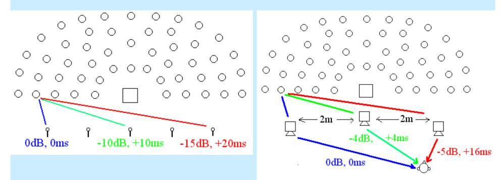
If you record with three widely spaced microphones, an instrument on the left will have high amplitude and time differences in the output signals. A listener on the far right will hear the instrument on the left. Now the orchestra spreads out across the entire loudspeaker basis.
